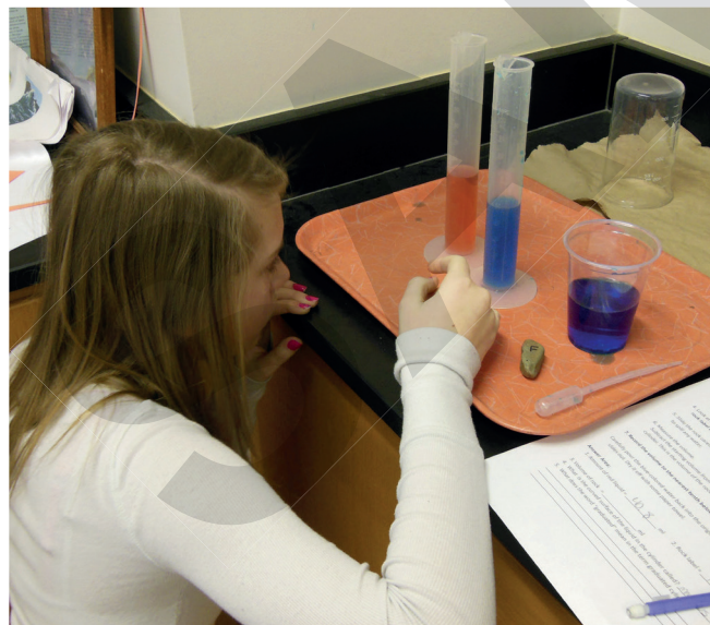
Figure 1.6: A student measuring the volume of a liquid. Her eyes are level with the scale so that she can accurately measure where the meniscus meets the scale.
